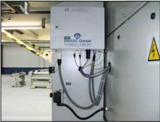
ESA 1000 Capacitance Free Power Supply integrated into a new rotogravure press
